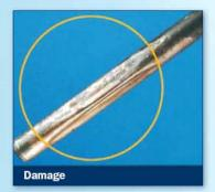
CAUSE: Abnormal damage or rust of the cartridge tube (accident damage, product abused or the presence of water inside strut housing).
