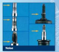
CAUSE: Knocking noise. Irregular damage of the piston rod stem thread.
