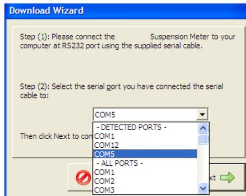
**Note:** For ordinary RS232 cable connection, it is very likely that the COM port would be COM1 or COM2. If you are using a USB cable, you need to select the COM port you would have figured out in **STEP 2**.
